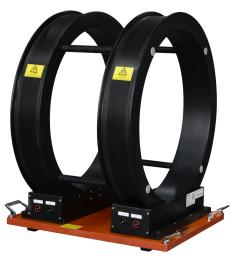
TYXH 06400 is used to produce d.c and alternating magnetic field from DC to 30 kHz together with appropriate signal source and compensation networks. Featured with large experimental area and good magnetic field uniformity, it can satisfy magnetic field susceptibility test requirement of various standard with frequency less than 30 kHz.
