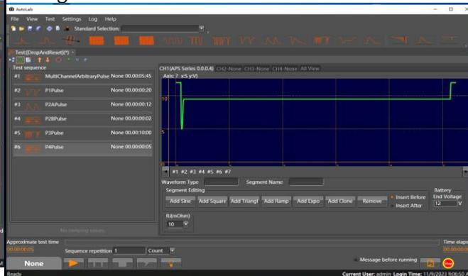
Multiple test step sequences and multiple test items can be added to a test, which is convenient for users to test a test sample, realize one-click testing, and test conveniently. For test parameters, Autolab also supports scheduling and setting multiple parameters to achieve iterative testing of parameters and avoid frequent parameter setting.
