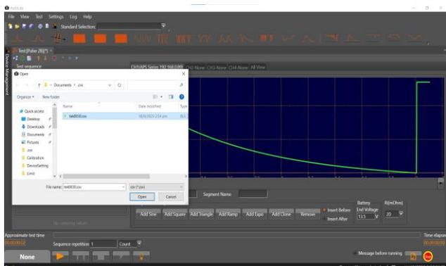
Supports reading the oscilloscope export format (. csv) file, users can also establish the waveform data file in Excel, after the system read (.csv) file, the corresponding waveform diagram is displayed on the interface, and the user can set the parameters and run the test.
