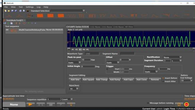
Support DC waveform, Harmonic, Sine wave, Sweep wave, Triangular wave, Square wave, Index wave, Frequency modulation / Amplitude modulation (FM/AM) sine wave standard waveforms, the above standard waveforms can be customized and edited into irregular waves and irregular arbitrary waves for testing, which fully explores the performance of the instrument and provides great scalability.
