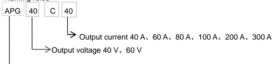
APG series are high power voltage failure simulator with current up to 300 A, impulse current 400 A, frequency up to 30 KHz
