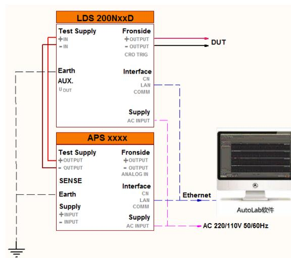
**Test Connecting Diagram 2:**
