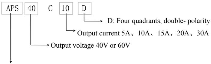
APS series can support external input signals, max. response frequency 250kHz, current up to 30A
