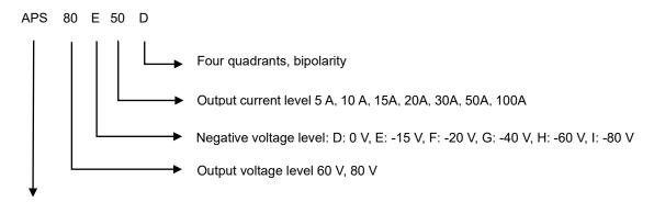
Type of simulator, support external input signal, Max. response frequency 300 kHz
