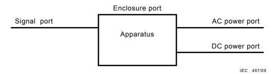
Figure 1 - Examples of ports
