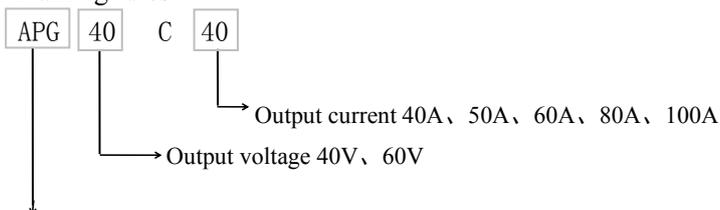
APG series are high power voltage failure simulator with current up to 100A, impulse current 200A, frequency up to 30KHz
